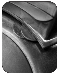
Double-stacked coins on the centrifugal disc.
