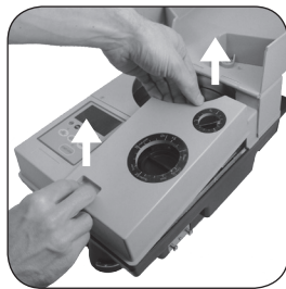
Removing the cover over the thickness and diameter dials.
