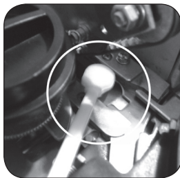
Cleaning the coin runway using a Clean Pro swab.
